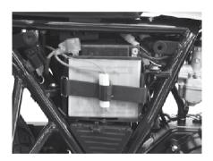
The fuse box is located inside the guard board on the right side of the chassis. A fuse is provided for the electrical system. In case of any trouble with the electrical system, check the fuse first. If the fuse is blown, replace it with the spare fuse (15A) in the fuse box.
