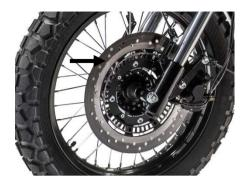
Check the brake pads to see if the wear is approaching the wear line. If wear exceeds the mark, the brake lining should be replaced with a new MASH approved parts.
