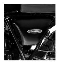
The tools box is right of side cover. To open the box, insert the ignition key and turn it clockwise and take down the box cover.
