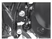
Rear brake light switch is located at the right side of chassis. Adjust the rear brake light switch as follows: Lift or lower the switch, so that, when the brake pedal is pressed, the lamp is lit before feeling a pressure.
