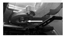
**4.** Tighten the oil drain ring and fill with fresh engine oil using the oil filler, before gently tightening the top cover.
