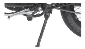
The vehicle is equipped with a side stand.
