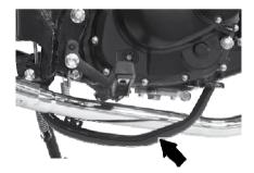
Press down this pedal to apply rear wheel brake. When operating the rear brake in this way, the rear brake indicator light is on.
