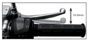
free stroke of brake handle: 10 - 20mm
