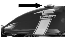
To open fuel tank cap, insert the key and turn it clockwise. Then, the fuel tank cap can be removed together with the key. To replace the cap, align the arrow on the cap and press the cap, together with the key, into the fuel tank cap hole until a click sound is heard. Then, remove the key.
