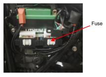
If the new fuse tube is broken again as soon as it is fitted on, it means that somewhere of the electric parts is shorted unexpectedly.
