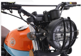
LED headlight with aluminum protection grill
