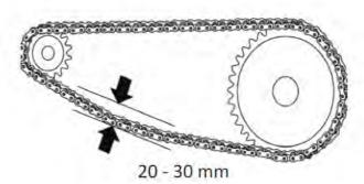
Note: When installing a new chain, it is necessary to check the pinion and crown. It is advisable to replace the chain kit.
